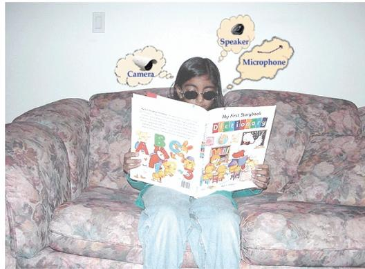
*Figure 1. Laura reads a book using a pair of glasses consisting of an integrated video camera and speakers wirelessly connected to a palm-size processing unit.*
