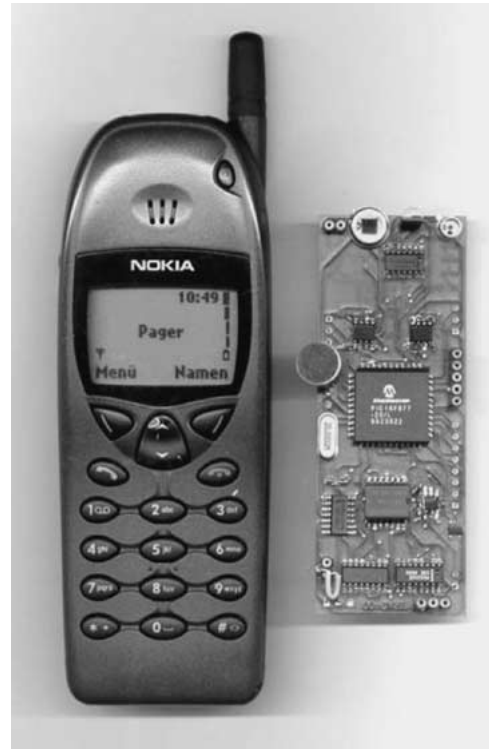
Figure 3. The TEA awareness device was implemented as self-contained module that can be connected via serial line to mobile host devices. The device has been applied for augmentation of mobile phones with context-awareness.
