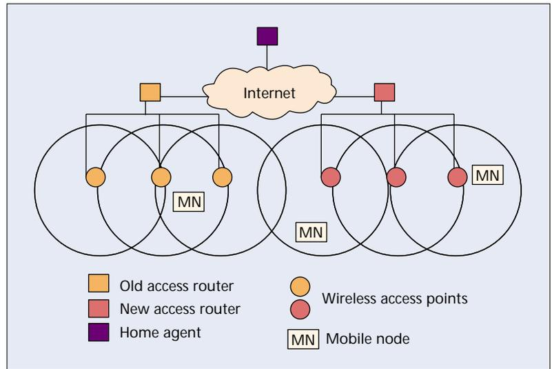
■ Figure 1. IPv6 wireless network architecture.
