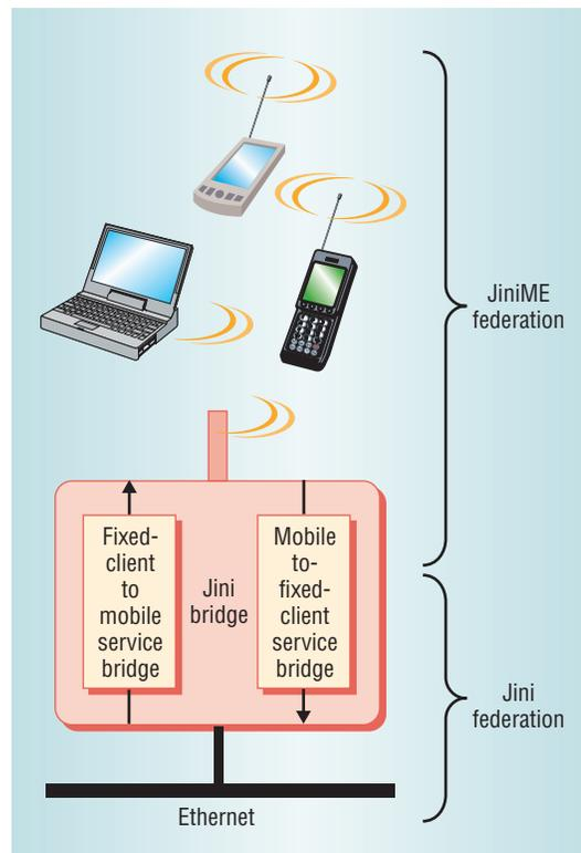
**Figure 3. JiniME federation with a Jini bridge to a standard Jini federation. A bridge component creates and maintains service objects for available wireless devices.**
