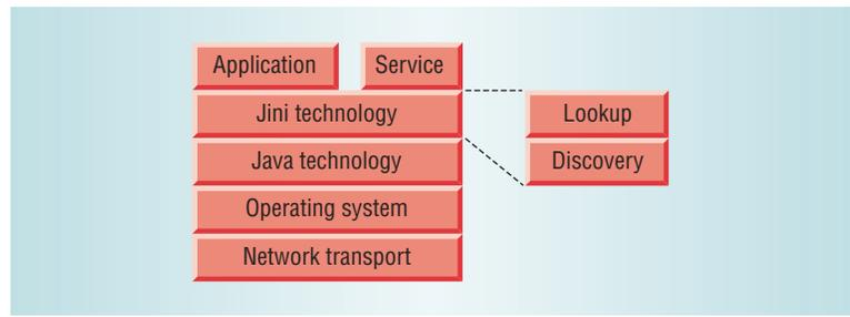
**Figure 1. A typical Jini network architecture implements the connection technology below the application layer and atop a Java platform.**
