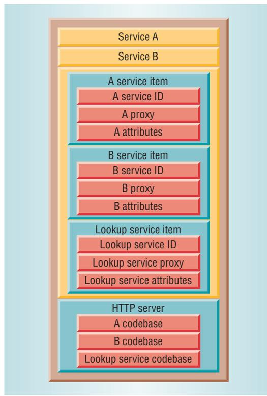
**Figure 4. Services in a JiniME-capable device. Each device houses its own lookup service and classfile server.**
