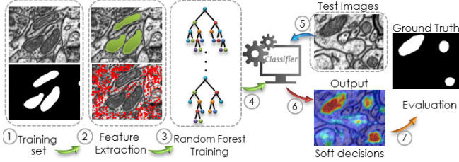
Fig. 2: Illustration of pixel classification framework: It depends on a random decision forest framework to provide a pixel wise probabilistic classification.
