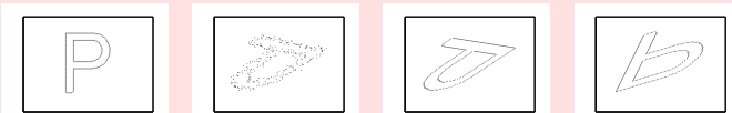
Pattern matching: original (a), transformed and noise added (b), recovered transformation with MSAP (c), and with MD (d).
