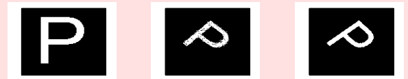
Image registration: original (a), transformed and noise added (noise=0.08) (b), recovered transformation ( \epsilon = 0.13 ) (c).
