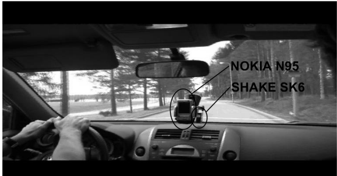
Figure 17. Test system mounted on the instrument panel in a vehicle.
